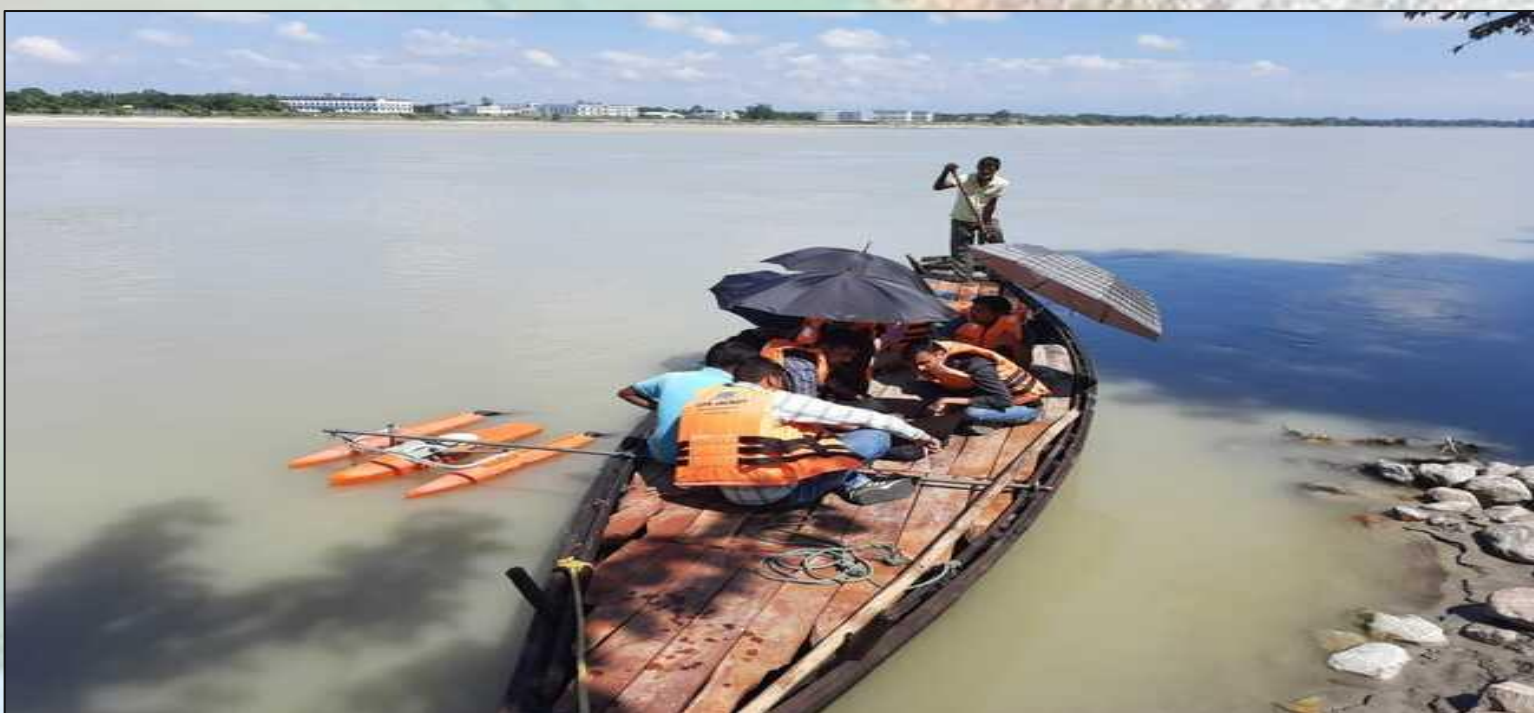
MEASUREMENT OF DISCHARGE THROUGH ADCP AT GHUGUMARI GDSQ SITE ON TORSIA RIVER, COOCHBEHAR, WEST BENGAL
