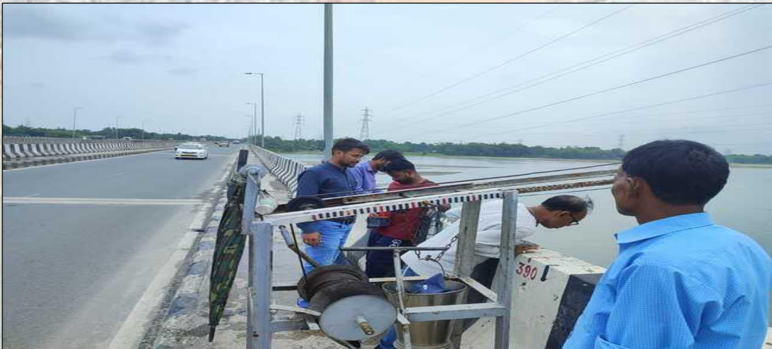
DISCHARGE OBSERVATION FROM BRIDGE AT NH-31 GDSQ SITE ON RIVER JALDHAKA, JALPAIGURI, WEST BENGAL
