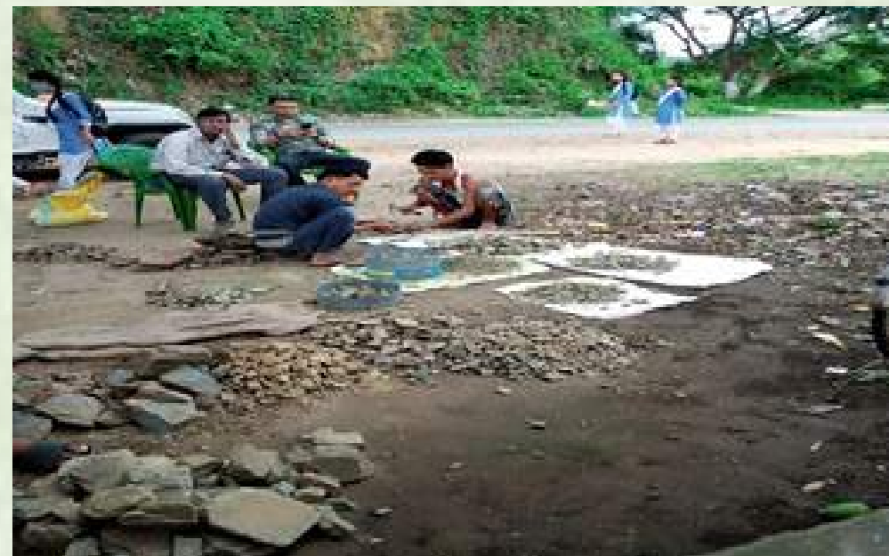
Breaking of Rocks collected from quarry site for lab testing for Construction Material for Haora and Champaicherra Dam Projects, West Tripura.
