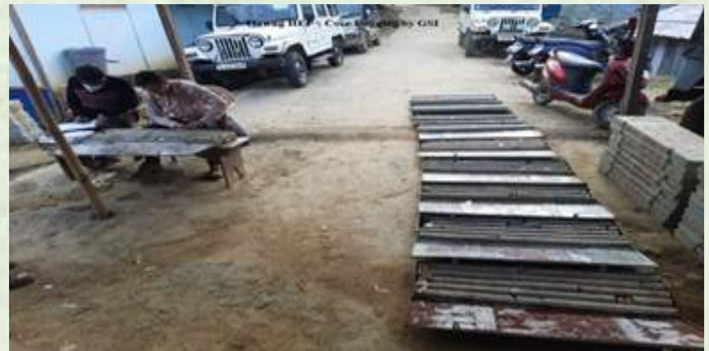
Core logged samples for analysis as part of subsurface investigation
